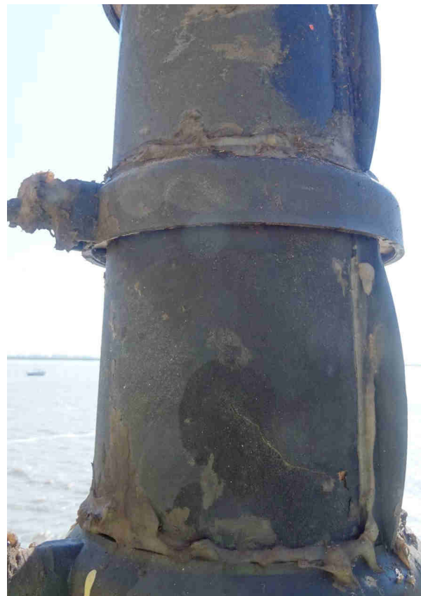
picture 3: sternlights, without wires but with silikon
